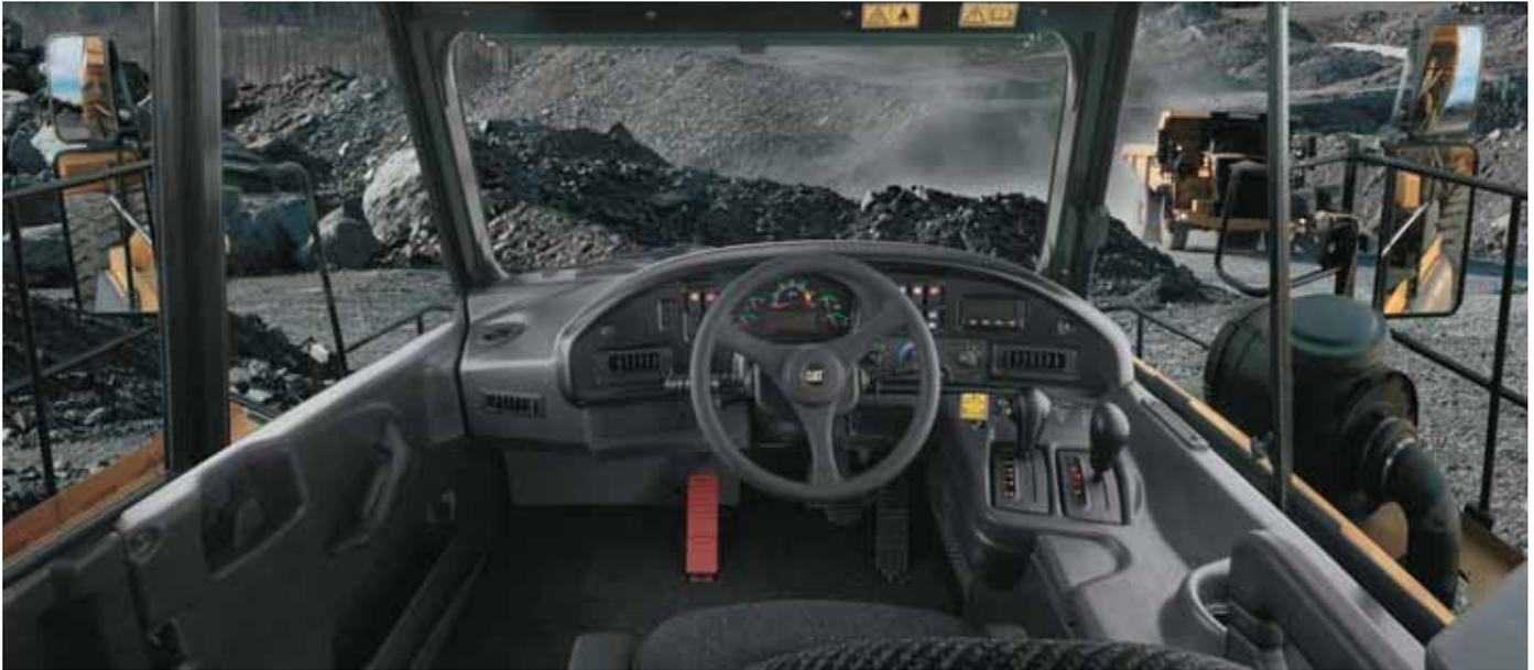
**All New Center-Mounted Cab.** Center cab positioning provides additional room and creates a walk-in-style cab. The new configuration allows the operator to easily enter and exit the cab. The cab environment offers a spacious surrounding, giving the operator the ability to stretch out and providing superior comfort for an entire operating shift. The operator seat is located on the right hand side of the cab with the trainer to the immediate left.
