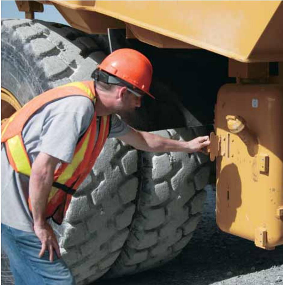
**Ground-Level Access.** All maintenance points have convenient ground level or platform access. Common engine service points are grouped on the right side of the engine for quick access. Two fuel filters come standard with the machine and the primary fuel filter includes a water separator. These filters are easy to change and are all spin-on/spin-off type.
