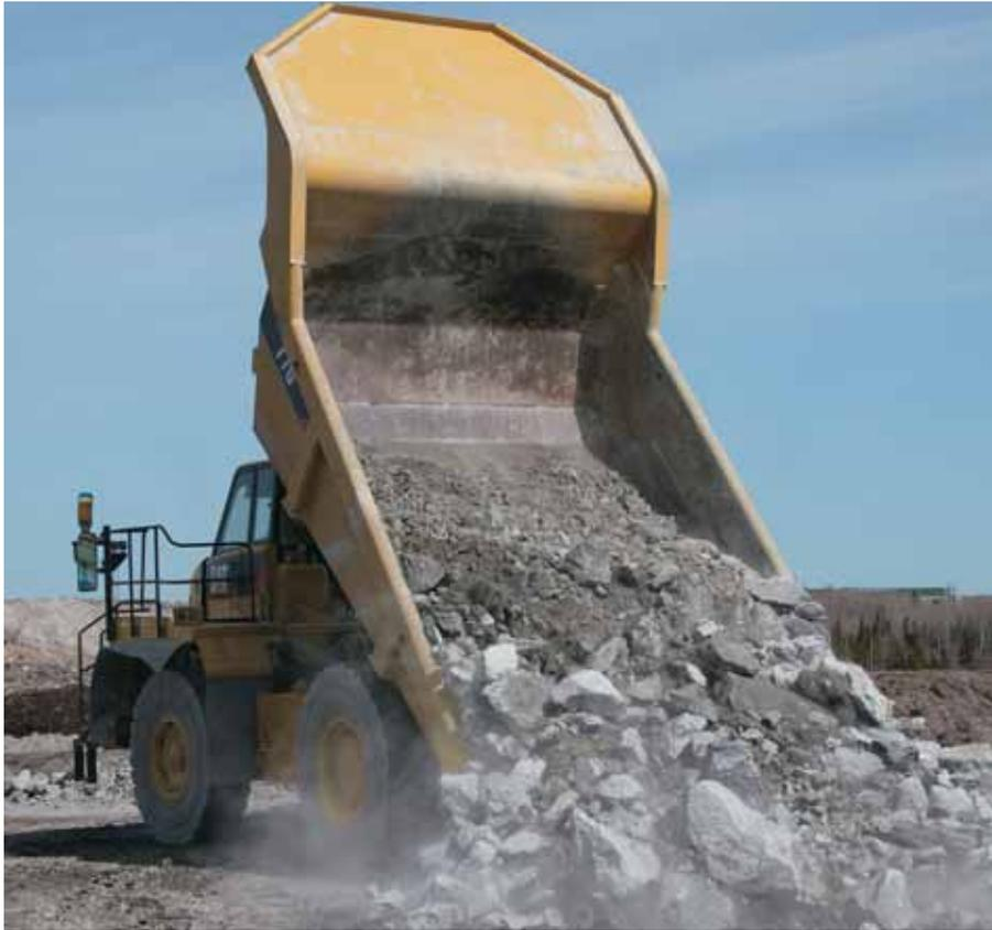
**Increased Body Capacities.** The 770 body capacity at 25.1 m<sup>3</sup> (32.9 yd<sup>3</sup>), has increased 3.5 percent over the 769 at 24.2 m<sup>3</sup> (31.7 yd<sup>3</sup>). Payloads are based on 1660 kg per LCM (2,800 lb per LCY) material.
