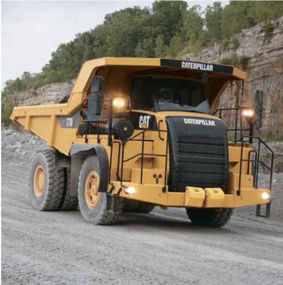
**Full Hydraulic Service Brake.** The 770 features a full hydraulic brake system, which offers significant improvements in reliability, response, control and serviceability versus an air-over hydraulic system. There are fewer components (part by part comparison), boosting reliability and streamlining maintenance.
