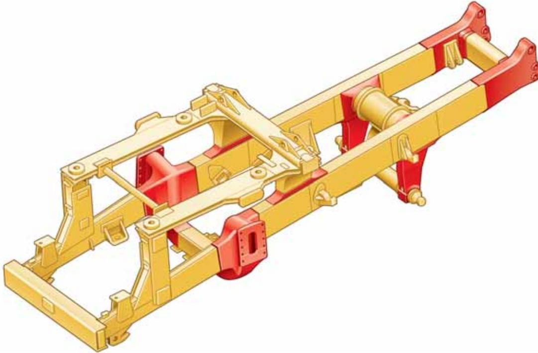
**Box-Section Design.** The 770 frame uses a box-section design, incorporating two forgings and 13 castings in high-stress areas with deep penetrating and continuous wrap-around welds to resist damage from twisting loads without adding extra weight.
