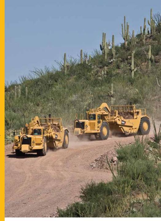
Quick loading, high travel speeds and the ability to load and dump on the run yield fast cycle times, allowing Cat® Wheel Tractor-Scrapers to deliver a high rate of productivity.
