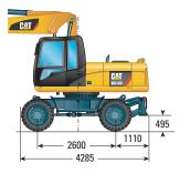
\*\* Maximum tire clearance with outrigger fully down
