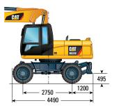
\* Maximum tire clearance with outrigger fully down
