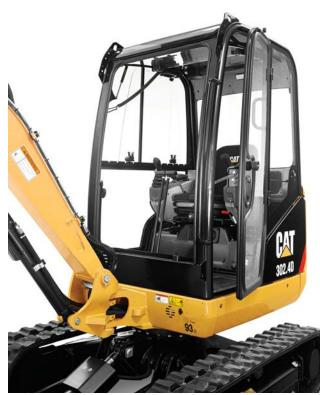
The Cat 302.4D cab is amongst the largest in the industry. The flat cab floor optimizes visibility and increases operator leg room. The ergonomic control layout provides a comfortable, highly productive workspace.
