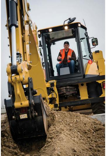
The 422F2 is fitted with mechanical controls providing low effort operation, with the ability to choose between ISO (Excavator) or SAE (Backhoe) control patterns. Providing easy and safe operation for operators of any experience or ability.
