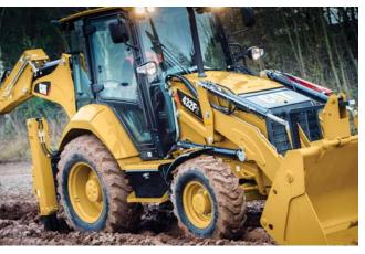
The 432F2 is fitted with pilot controls providing low effort operation, with the ability to switch between ISO (Excavator) or SAE (Backhoe) control patterns with the press of a button. Providing easy and safe operation for operators of any experience or ability.
