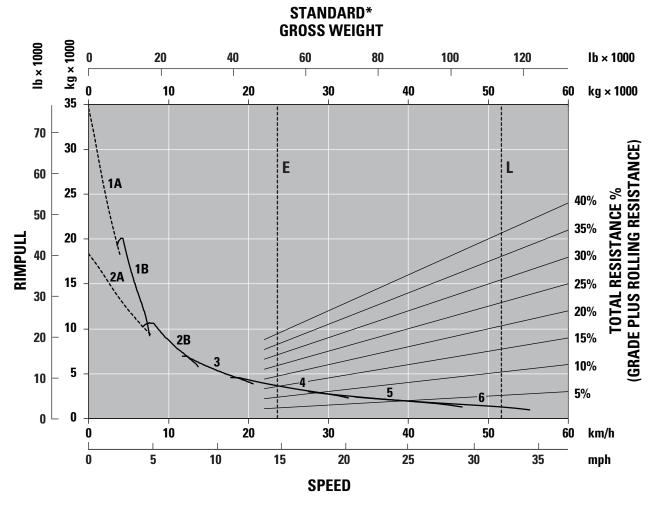
1A – 1st Gear (Converter Drive) 1B – 1st Gear (Direct Drive)
