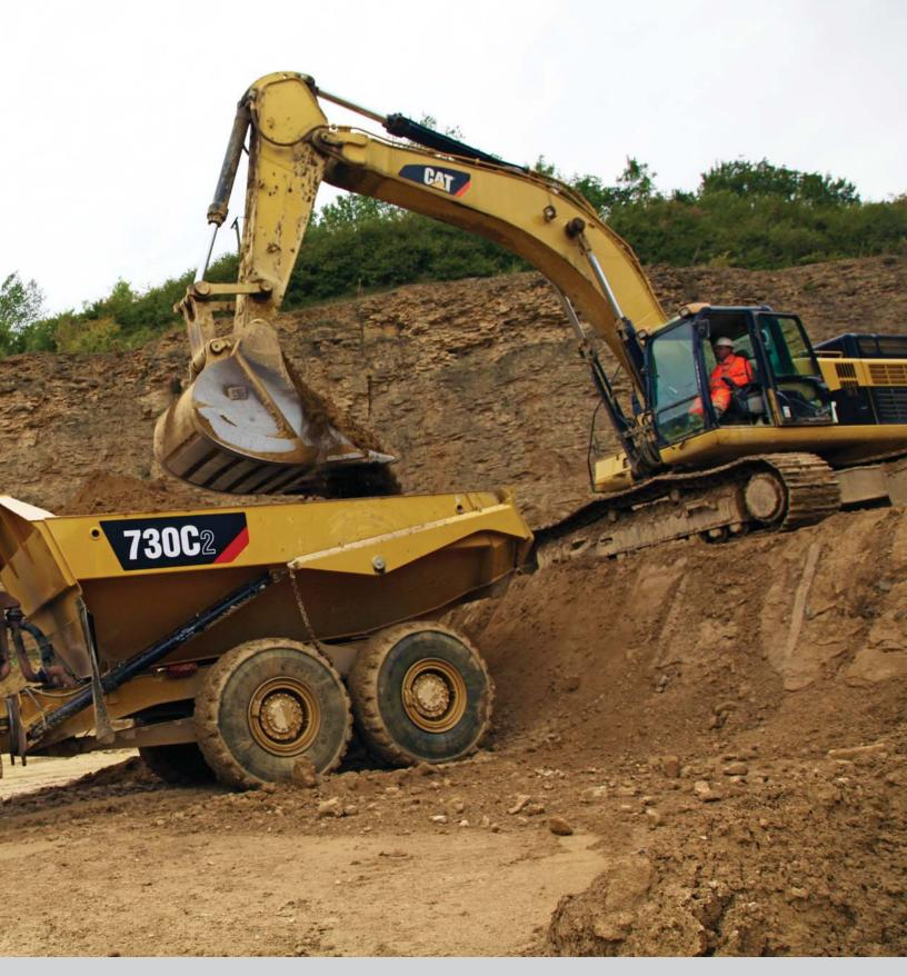
The Cat 730C2, with a 17  $m^3$  (23 yd<sup>3</sup>) 28 tonnes (31 tons) capacity, offers demonstrated reliability and durability, high performance and productivity, superior operator comfort and lower operating costs.
