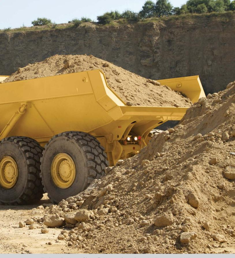
The Cat 735C with a 22 m³ (28.7 yd³) 32.7 tonnes (36 tons) capacity offers proven reliability, durability, high productivity, superior operator comfort and lower operating costs.
