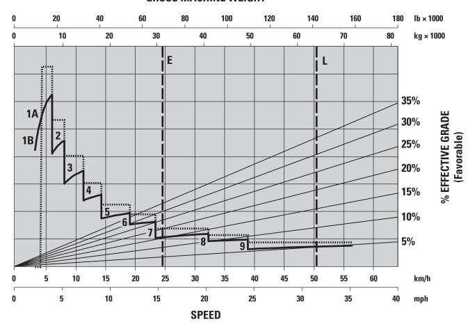
1A – 1st Gear (Converter Drive)
