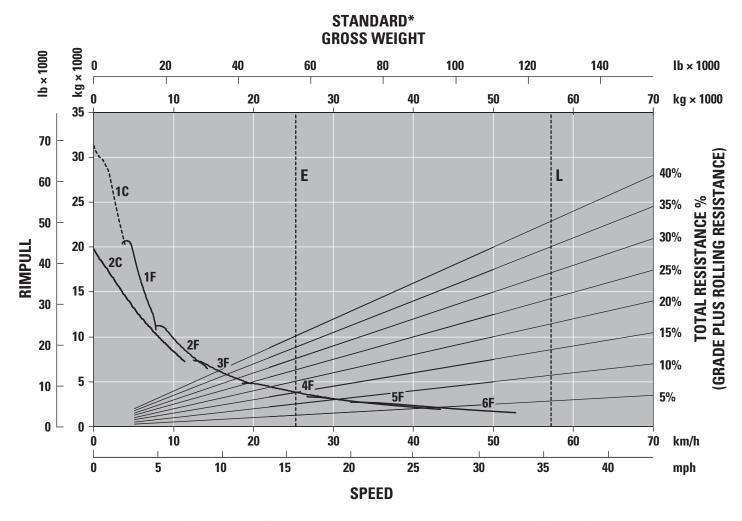
1C – 1st Gear (Converter Drive)
