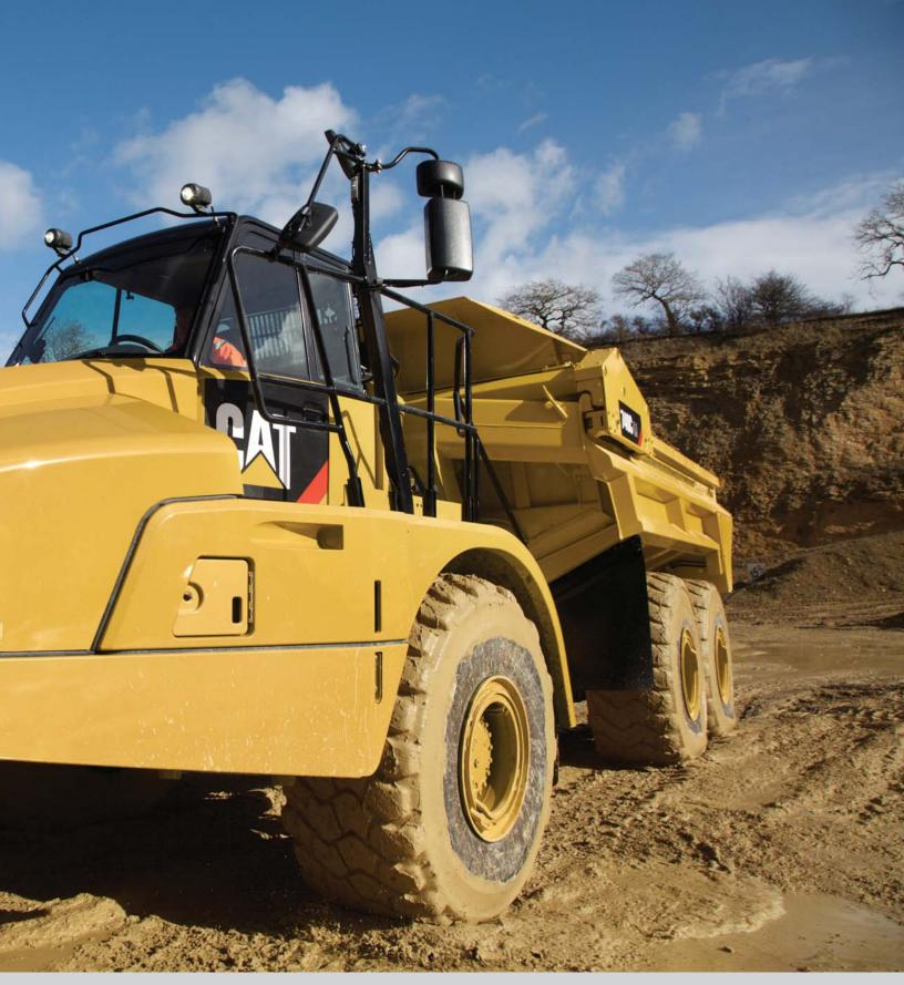
The Cat 740C EJ with a 23 m<sup>3</sup> (30.1 yd<sup>3</sup>) 38 tonnes (42 ton) capacity offers proven reliability, durability, high productivity, superior operator comfort and lower operating costs.
