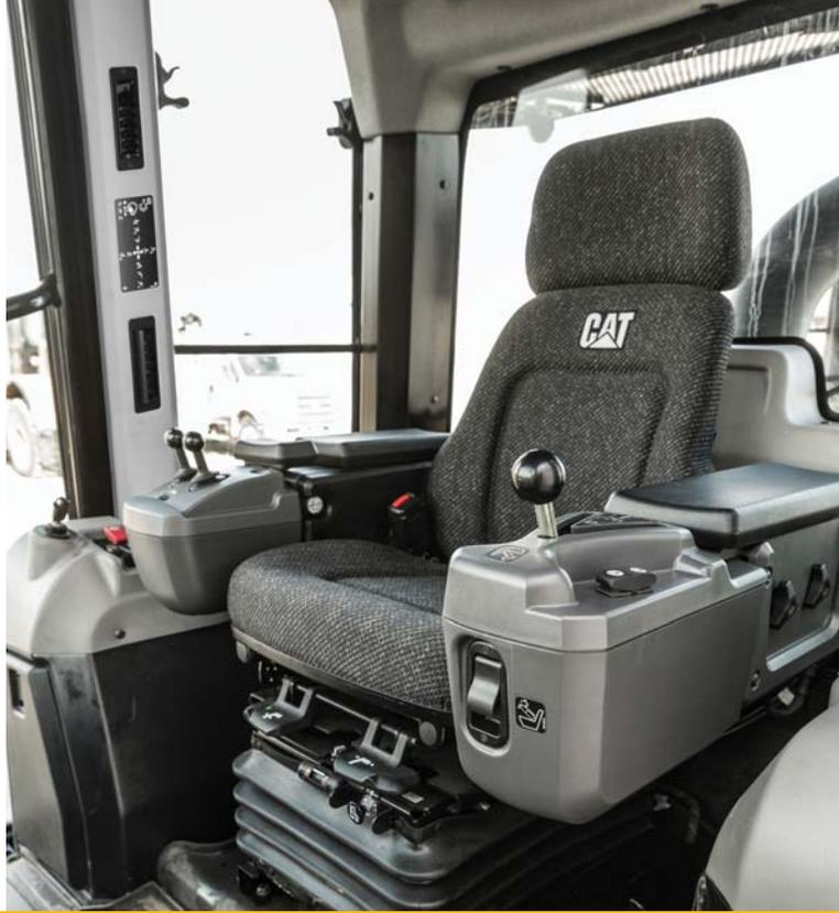
Updated cab gives operators added comforts like adjustable armrests and controls, improved air conditioning system and a heated/ventilated seat option. A new LCD operator interface makes it simple to customize machine performance features and to view machine operating and service information.
