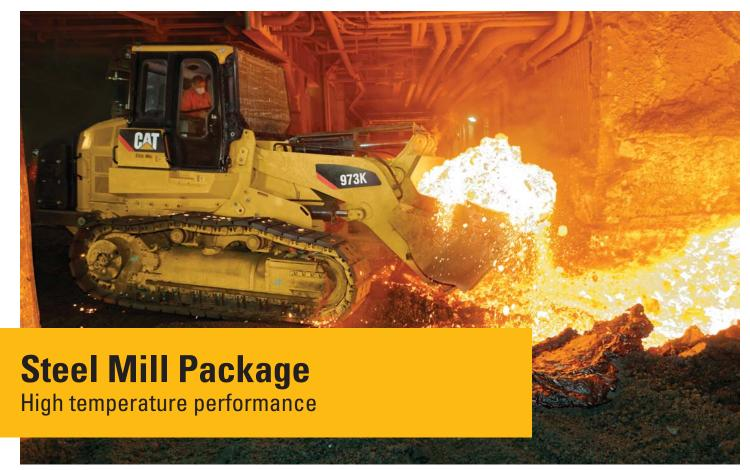
Factory designed and installed features equip your loader for the extreme heat and harsh conditions of steel mill work. Maneuverability, visibility and the breakout force needed for fast cycle times make track loaders a rugged and efficient choice for handling slag.
