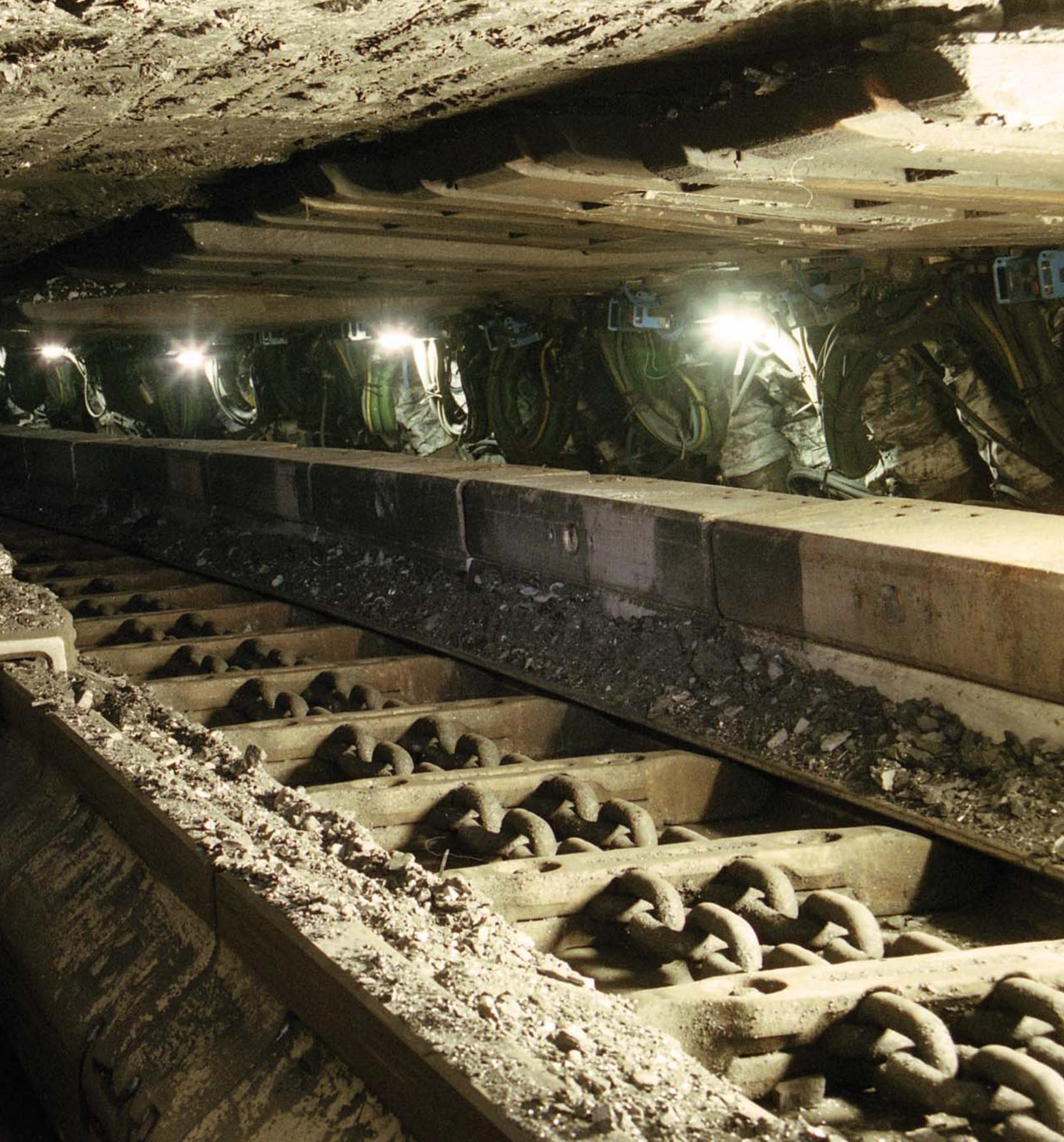
The Gleithobel Plow System GH1600 was specifically developed for very hard coal and high productivity by doubling the installed power of the GH800 to 1600 kW (1,080 hp). It can be used in seams from approximately 1.0 m (39 in) up to 2.53 m (91 in) with a portal arm.
