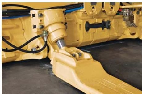
Effective plow horizon control is necessary to cope with undulations in the coal seam. Following the coal seam minimizes cutting of adjacent rock strata and the associated preparation costs, reduces cutting tool (bit) consumption and reduces power consumption while maximizing seam recovery. Caterpillar has developed an outrigger steering system for vertical horizon control with hydraulic cylinders between the gob-side of the AFC and the roof support's relay bar.
