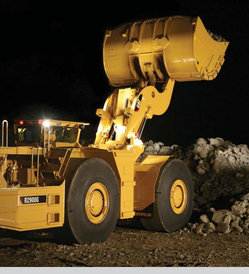
The R2900G underground loader is designed for high production, low cost-per-ton loading and tramming in underground mining applications. Compact design with agile performance, rugged construction and simplified maintenance ensures excellent productivity, long life and low operating costs.
