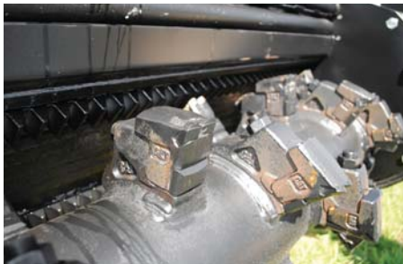
Single bolt carbide tooth retention
