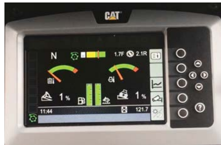
Drum direction and speed bar
