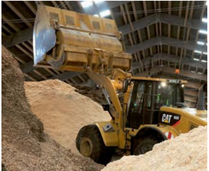
The wood-chip bucket, supplied by local Cat dealer Avesco, has a capacity of 12 cubic metres – it's so huge that a camera – similar to a submarine periscope – is needed to safely operate the loader.
