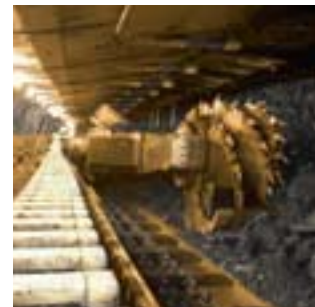
The Cat EL4000 shearer effortlessly cuts coal from an underground seam.
