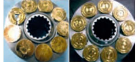
The test with conventional oil was terminated after 178 hours due to catastrophic failure caused by the slipper wear.
