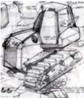
A preliminary sketch for the D7E highlights a new approach to cab design offering substantially improved ergonomics.
