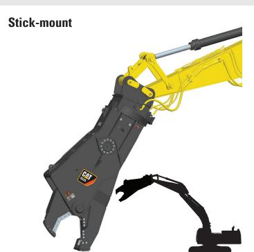
Cat Shears are commonly stick-mounted for use in demolition applications where reach is critical.
