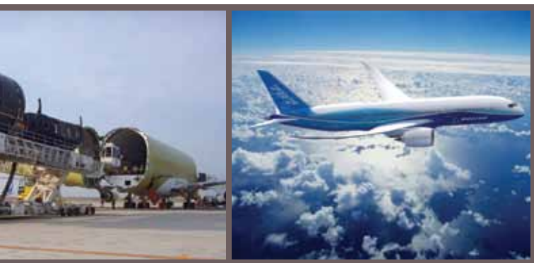
The DBL-110 (Dream Big Loader), shown at left, is used to load Boeing's Dreamlifter 747 aircraft, shown in center photo. The DBL is powered by a pair of Cat® C9 ACERT®. The Dreamlifter is a large, specially-designed aircraft that carries airplane parts back to the Boeing assembly plant. This plant assembles Boeing 787 Dreamliner aircraft, shown in right photo.
