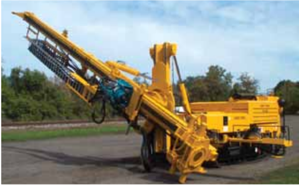
(Left photo) The DK720, powered by Cat® C7 ACERT®, incorporates a rotary bearing and a zoom-boom mast connection for micro-pile and anchor drilling. The sturdy mast structure and hinge support allow the DK720 to be mounted with some of the industry's largest rotators and drifters.
