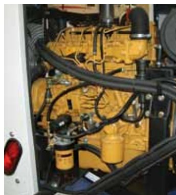
The Cat® C4.4 ACERT® is the standard power source for both the GS 700 and the GS 1400 deicing systems.
