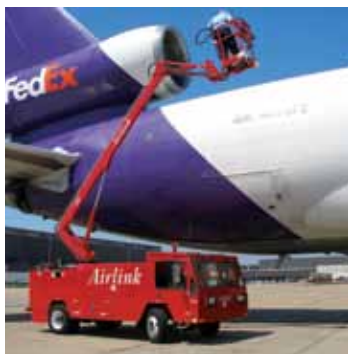
The GS 700 (shown at left) and the GS 1400 (above) can deice virtually all craft smaller than a Boeing 727.
