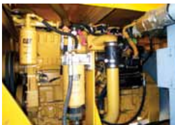
Cat® C7 ACERT® provides 215 hp (160 kW) at 2,200 rpm in the Davey Drill DK720 and 240 hp (179 kW) at 2,200 rpm in the DK820 drill rig. Both machines also use additional Cat components such as sleeve bearings, seals and engine hold-down latches.
