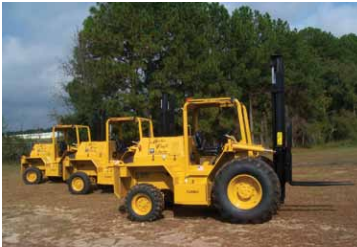
The C-Series rough terrain forklifts are powered by Cat® C4.4 ACERT®. The engines are paired with fully synchromesh Caterpillar power shuttle transmissions with a torque converter and Cat drive axle.
