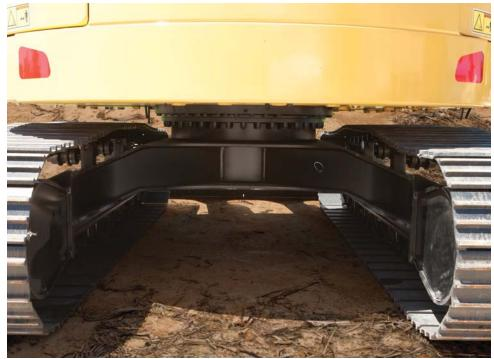
The 315F L is a well-built machine designed to give you a very long service life. The upper frame has mountings made specifically to support the heavy-duty cab; it's also reinforced around key areas that take on stress like the boom foot and skirt. Massive bolts are used to attach the track frames to the body, and additional bolts are used throughout to increase the machine's digging force, which leads to more productivity for you.
