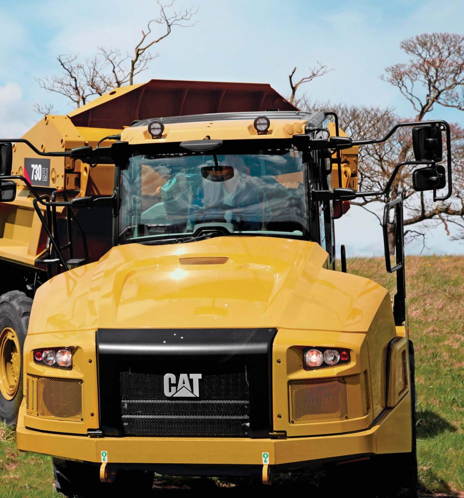
**The Cat 730 EJ with a 16.9 m<sup>3</sup> (22.1 yd<sup>3</sup>)/27.1 tonnes (30 tons) capacity, offers demonstrated reliability and durability, high performance and productivity and a new world-class cab to improve operator comfort and ease of operation.**
