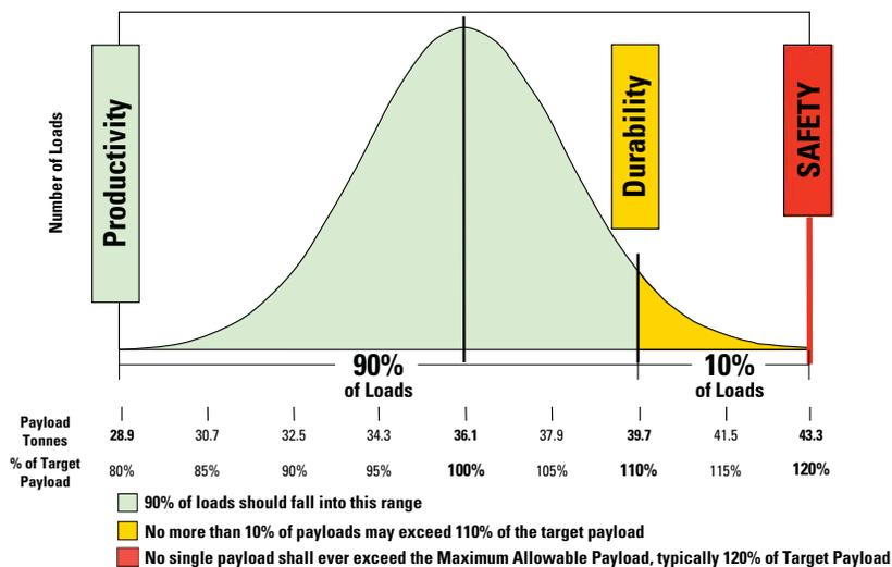
Consistently overloading any truck will affect component life, reduce tire life, increase haul road maintenance and most importantly negatively impact your cost of doing business. Caterpillar's 10/10/20 payload guidelines are in place to help you maximize the availability of your trucks and manage your hauling costs.
