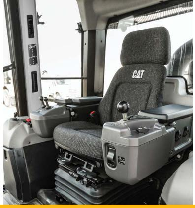
Updated cab gives operators added comforts like adjustable armrests and controls, improved air conditioning system and a heated/ventilated seat option. A new LCD operator interface makes it simple to customize machine performance features and to view machine operating and service information.
