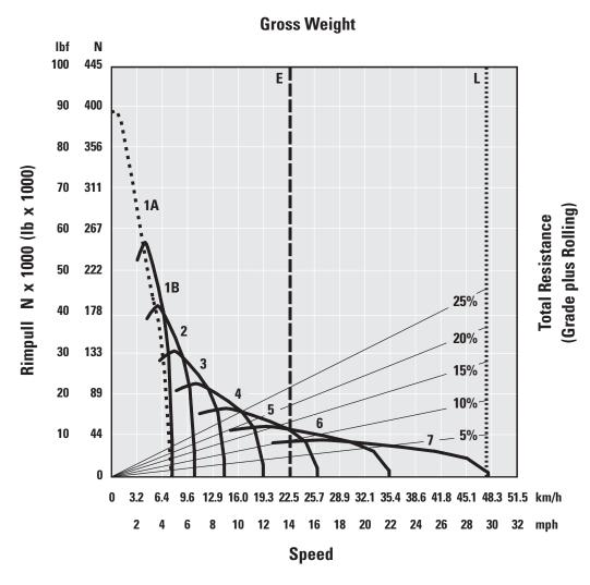
1A – 1st Gear Torque Converter Drive
