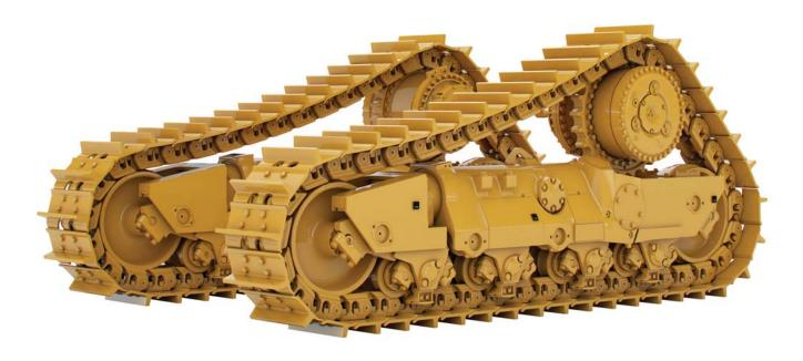
The elevated sprocket and fully suspended undercarriage work together, increasing traction while creating a smoother ride for your operators. The elevated sprocket design transfers implement shock loads to the mainframe, so final drives, axles and steering components are isolated from harsh impacts. These benefits translate into higher production and longer component life.
