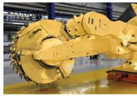
Cat shearers can be supplied with an optional rugged coal sizer, currently with up to 200 kW (268 hp) of installed power for maximum productivity in high seams or difficult mining conditions. The coal sizer can be ordered separately for installation during rebuild or overhaul.
