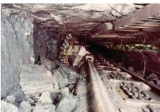
Effective plow horizon control is necessary to cope with undulations in the coal seam. Following the coal seam minimizes cutting of adjacent rock strata and the associated preparation costs, reduces cutting tool (bit) consumption and reduces power consumption while maximizing seam recovery. Caterpillar has developed an outrigger steering system for vertical horizon control with hydraulic cylinders between the gob-side of the AFC and the roof support's relay bar.
