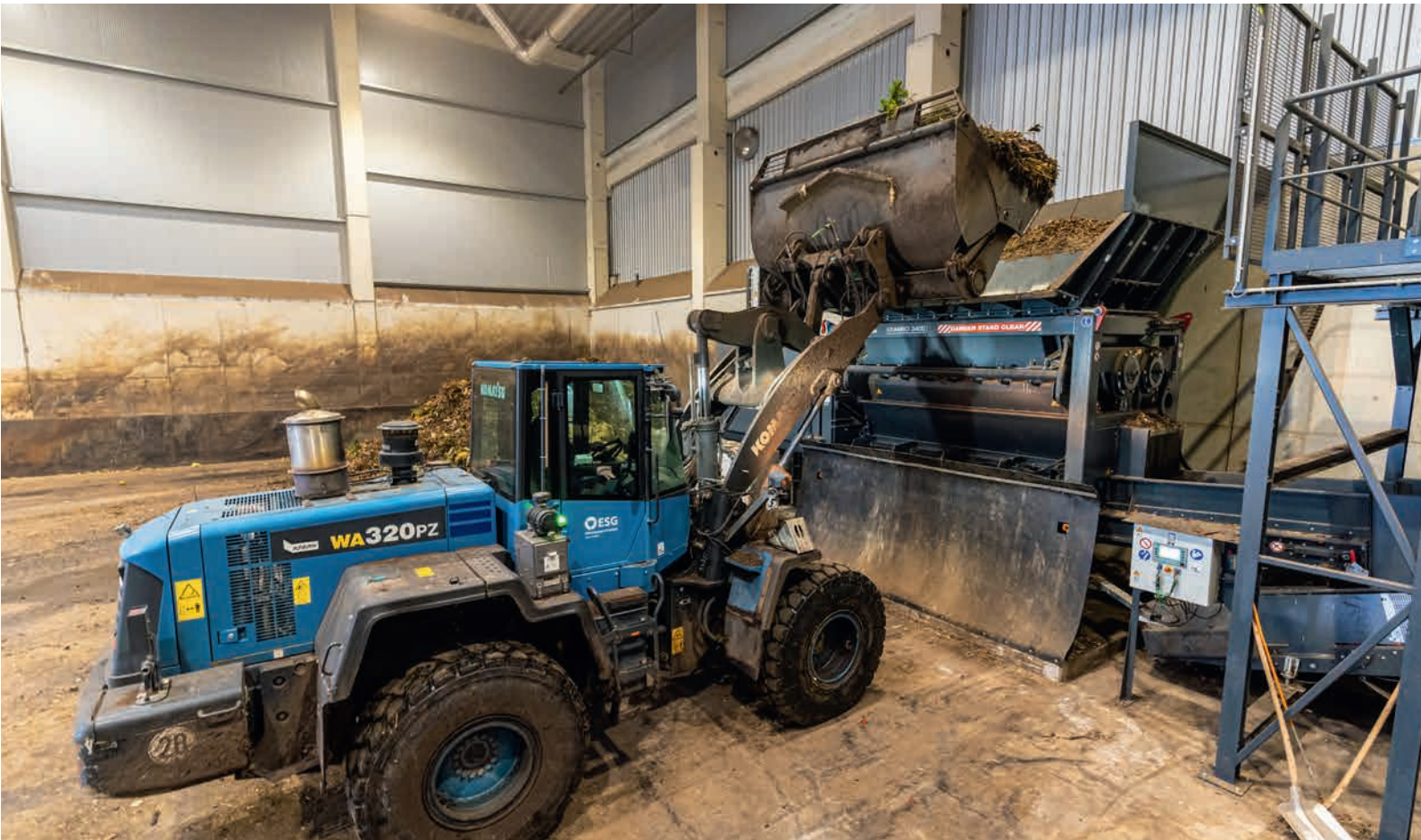
As a low-speed shredder, the Crambo gives very gentle opening of bagged organic waste.
