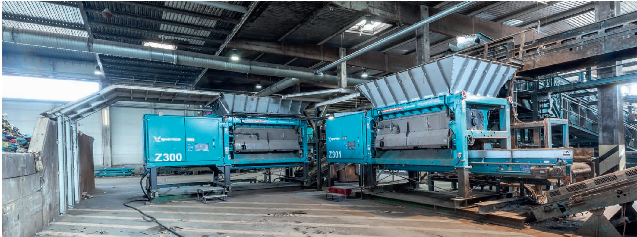
Dependable shredding and dosing – the tasks of the Terminators. Every day several hundred tonnes of residual waste pass through the shredders.
