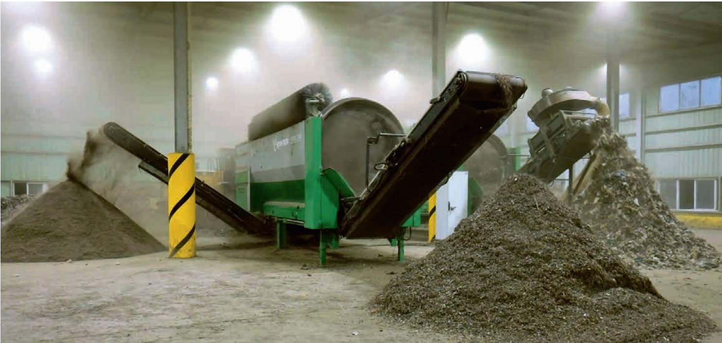
Final conditioning of the compost is done by drum screening and wind sifting.
