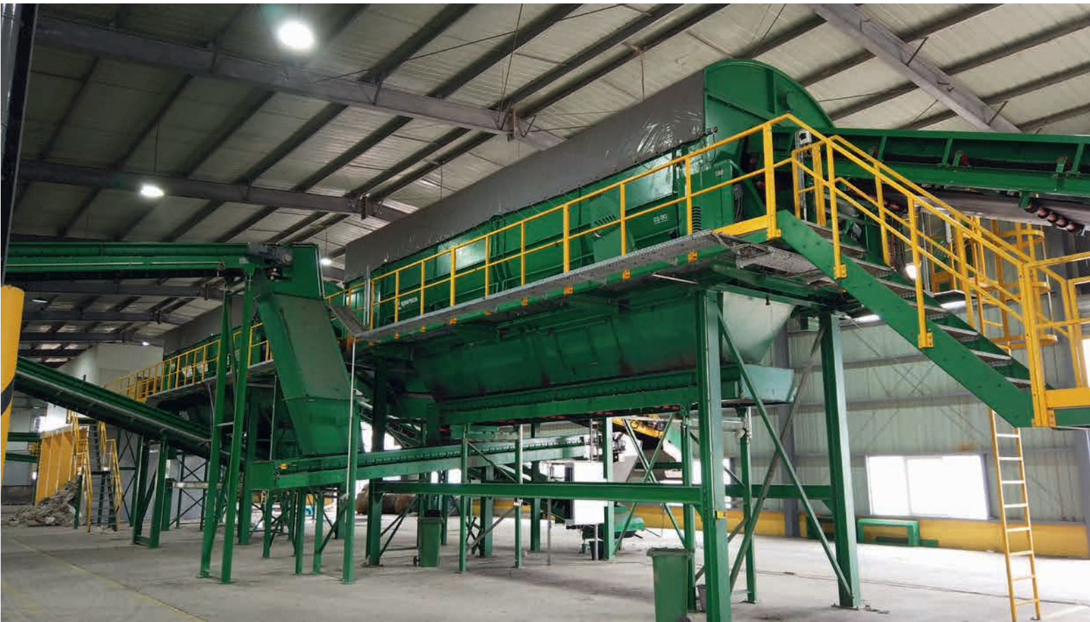
First comes mechanical preparation with separation of the recyclables, then comes biological treatment. The organics are first opened up and then composted in windrows. Subsequent fine processing provides high compost quality.
