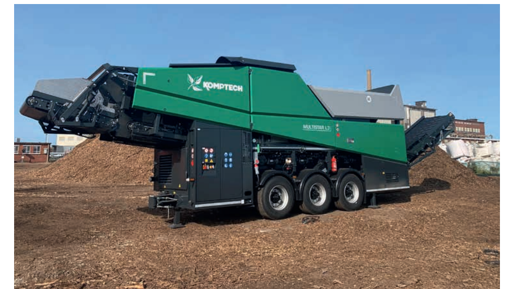
With 40 percent more screening area, the extended coarse screen deck is ideal for screening biomass. For transportation the extension is folded down.
