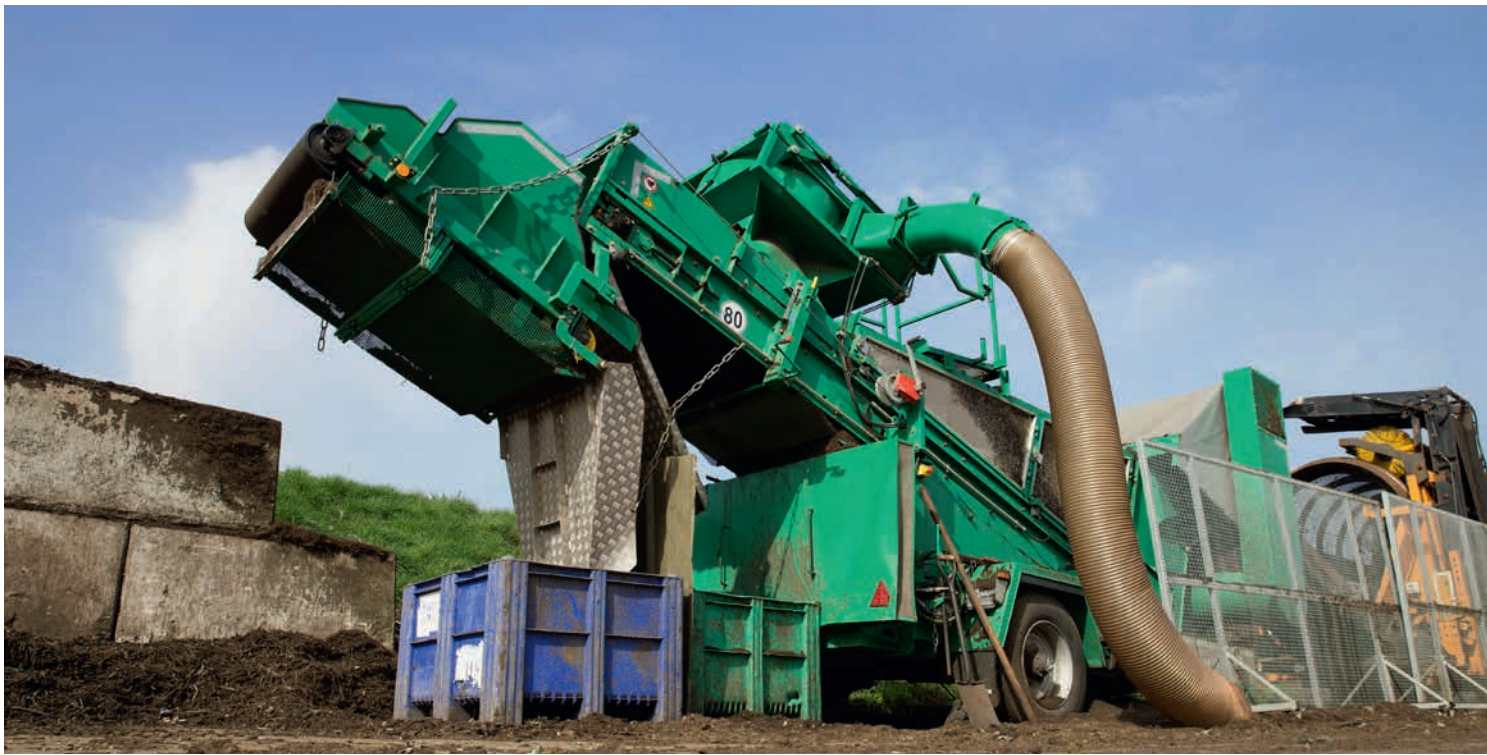
Windsifting by Hurrikan is an important part of the process.
