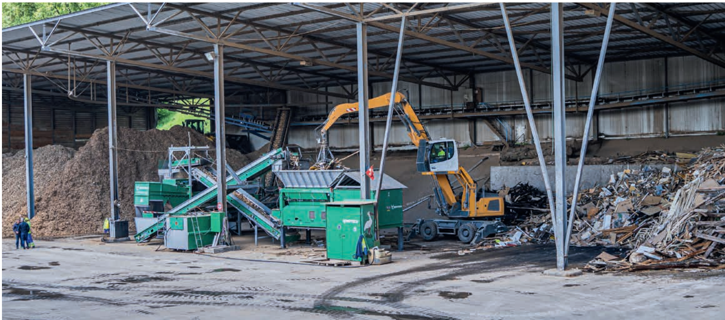
On the right the input material, on the left the finished fuel, in between the compact processing system
