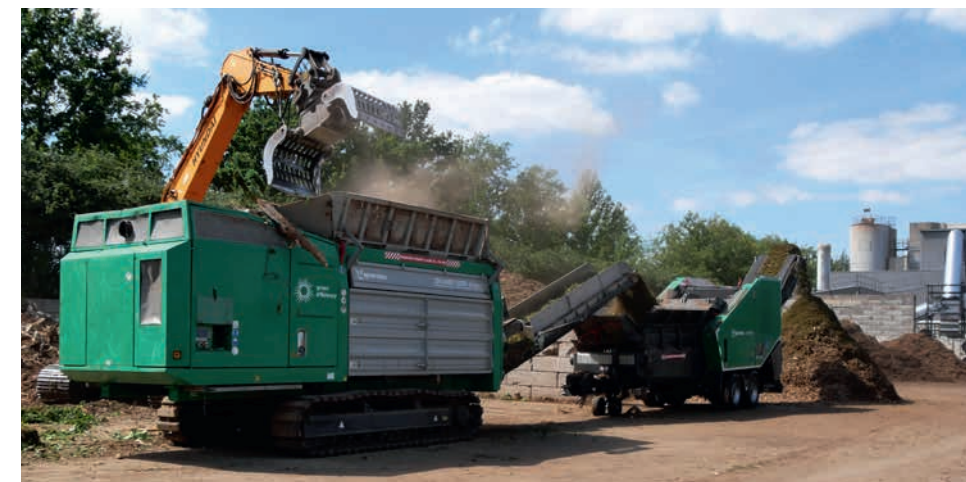
A robust duo for rootstocks, used wood and green cuttings with possible contraries: Crambo as pre-shredder and Axtor as post-shredder
