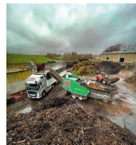
The Axtor has a 4.5 meter cone height, making direct filling of trailers possible.
