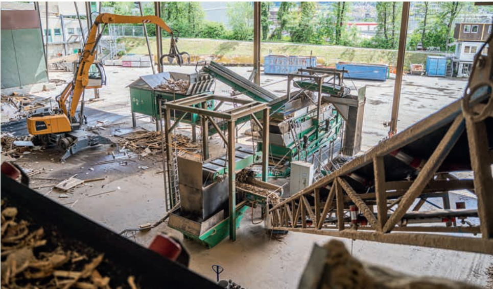
A conveyor system takes the fuel directly to the storage hopper of the cogeneration plant.
