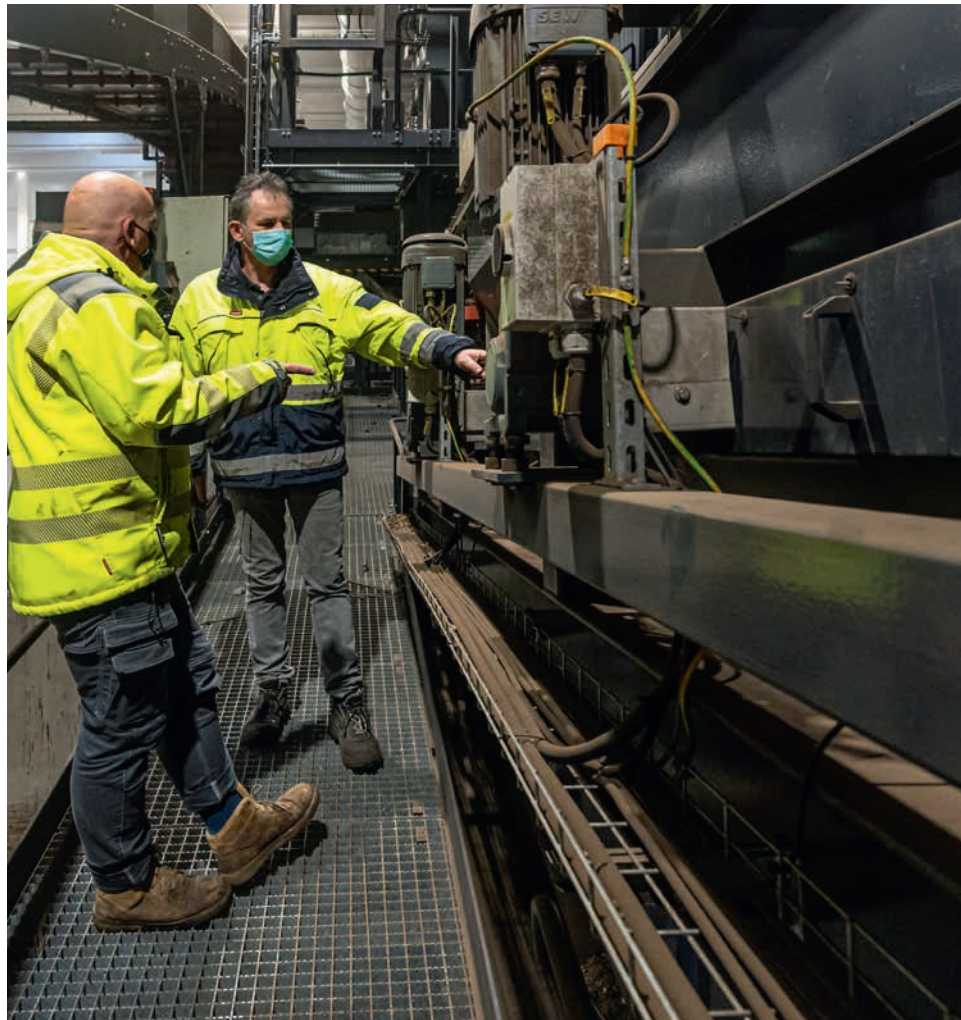
The electric motors with frequency converters make the star screen precisely adjustable.
