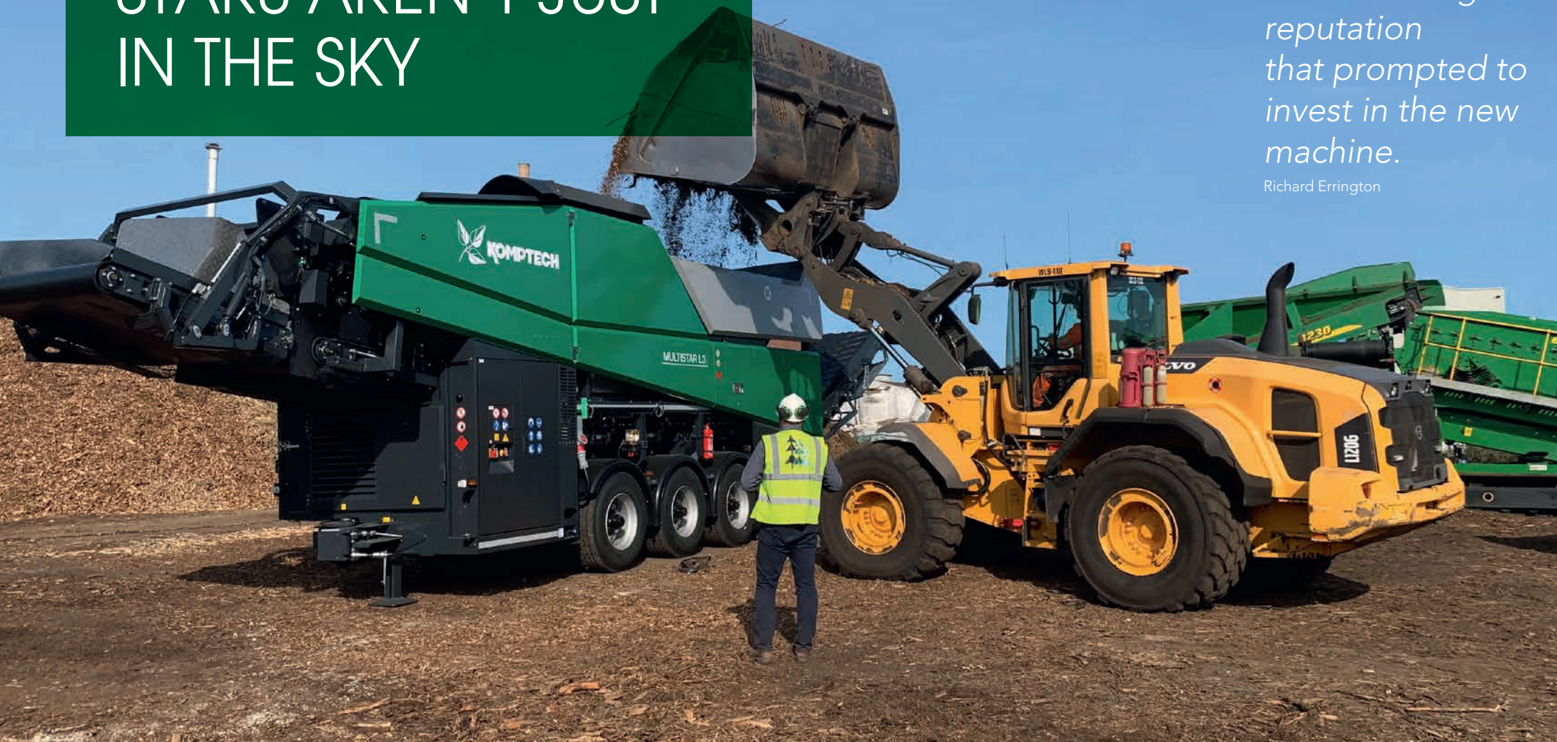
Large wheel loaders welcome! The hopper of the Multistar L3 holds seven cubic metres.
