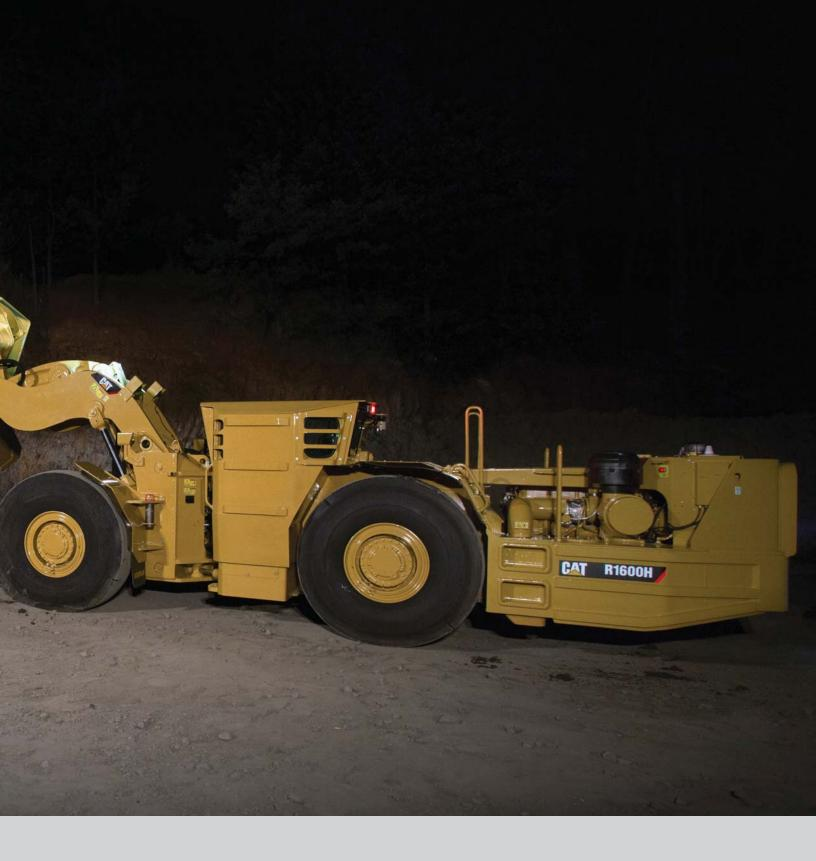
The R1600H underground loader is well matched to the AD30 underground truck for a loader and truck combination. The R1600H can easily load the AD30 truck fitted with a dump body or ejector body configuration using a standard dump bucket or if restricted by height the ejector bucket option could be used on the loader.
