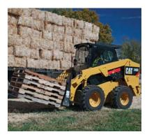
Cat pallet forks are used for a variety of material handling needs, such as moving bulky or palletized materials on construction and industrial sites, handling bagged fertilizer and seed at landscaping and nursery sites, and similar jobs.
