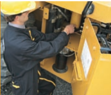
Daily service is made easy with ground-level service points which group together all the electronics, grease and pressure points and filters.
