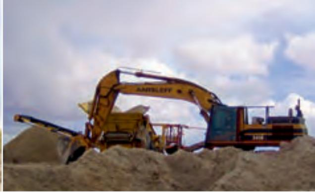
Below: The Cat 345B hydraulic excavator was fitted with a special cover, this protected the operator in the event of a mine exploding.
