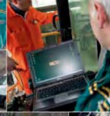
Bechelli and CGT technician Stefano Bastianoni have installed fuel flow meters supplied by Caterpillar from the USA, data recording equipment and a wireless communications adaptor in the machine to try to track down the source of the problem. Paolo is here to study the results and make repair recommendations. Within two hours of his arrival, the problem has been diagnosed, a remedy found, and the 992G is back at work in the quarry.
