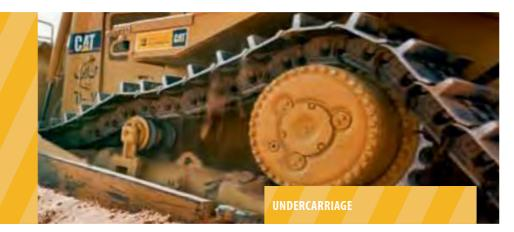
Did you know that on a track-type tractor, the undercarriage can represent as much as 50 percent of machine maintenance costs? Here we outline conditions and situations affecting the undercarriage and highlight ways to help you slow or reduce wear.
