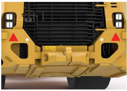
We've integrated more tie down and lift points to this machine to help drop it down a mine shaft. The new optional tow hook is bolted on for quick removal and installation.
