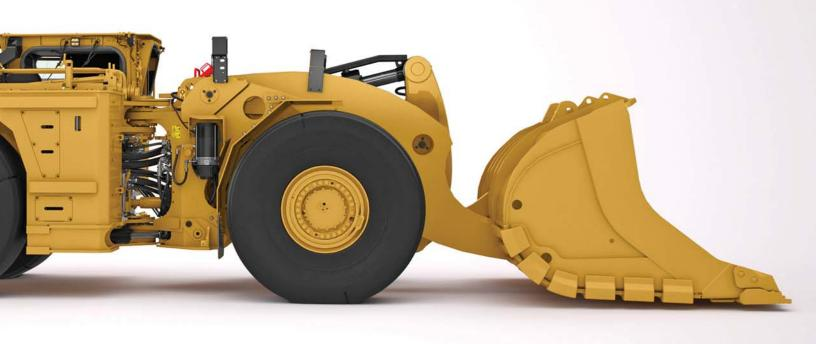
Our goal for the redesign of the R1700 was simple; add value, power and performance with safety at its core. With each cycle, the R1700 hauls 20 percent more payload, it loads, climbs, hauls and dumps quicker. It features three engine emission options that can be tailored to your mine's ventilation requirements. The R1700 is a powerful new tool for mining.
